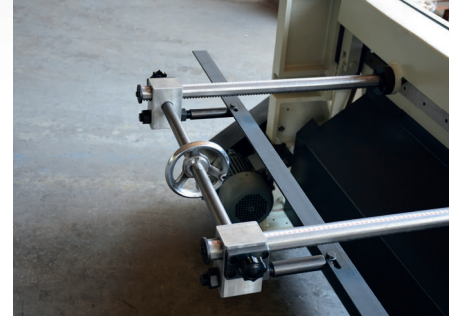
Arka Dayama 600 mm Back Gauge 600mm
