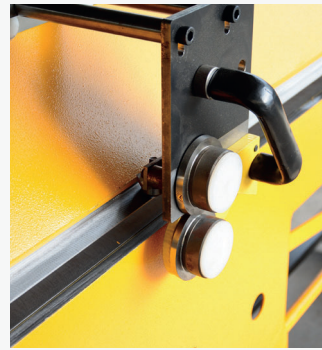
Standart Kesme aparatı Standard Cutting attachment
