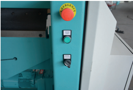
Otomatik ( Manuel Büküm) Automatic ( Manual Bending)
