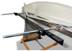
500mm e kadar arka dayama Back Gauge up-to 500mm
