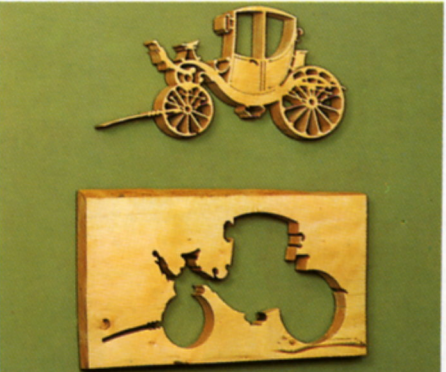
The POLYCUT-3 changed this 1\frac{1}{2} " thick beech plate into this decorative antique coach (20 x 9") quickly, precisely, and without blade breakage.
