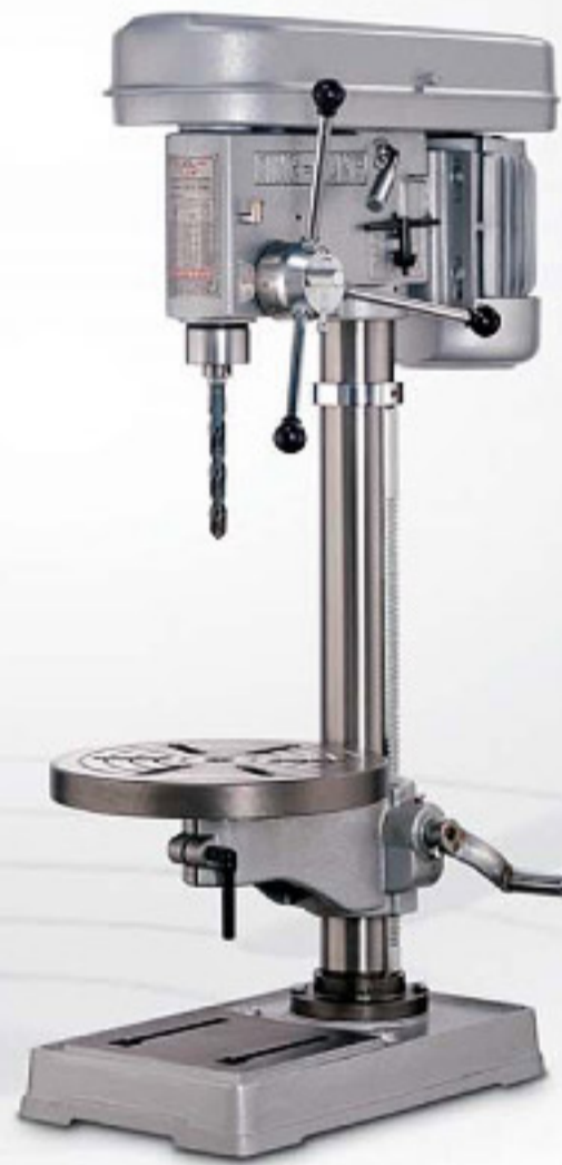
KSD-16 5/8" Drilling machine 鑽床
