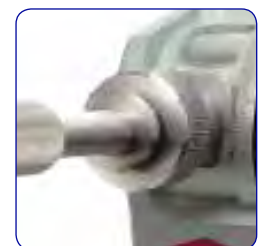
Eccentric plate triples the use of the diamond wheel
