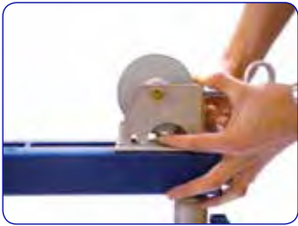
1. Lift quick release tab
