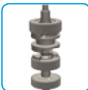
Four stage gear 120/180/320/440RPM
