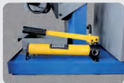
液压调高 Hydraulic height adjustment
