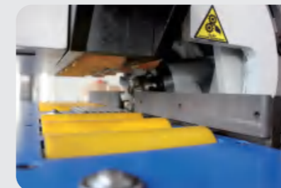
橡胶轮压紧 Clamp is rubber roller
