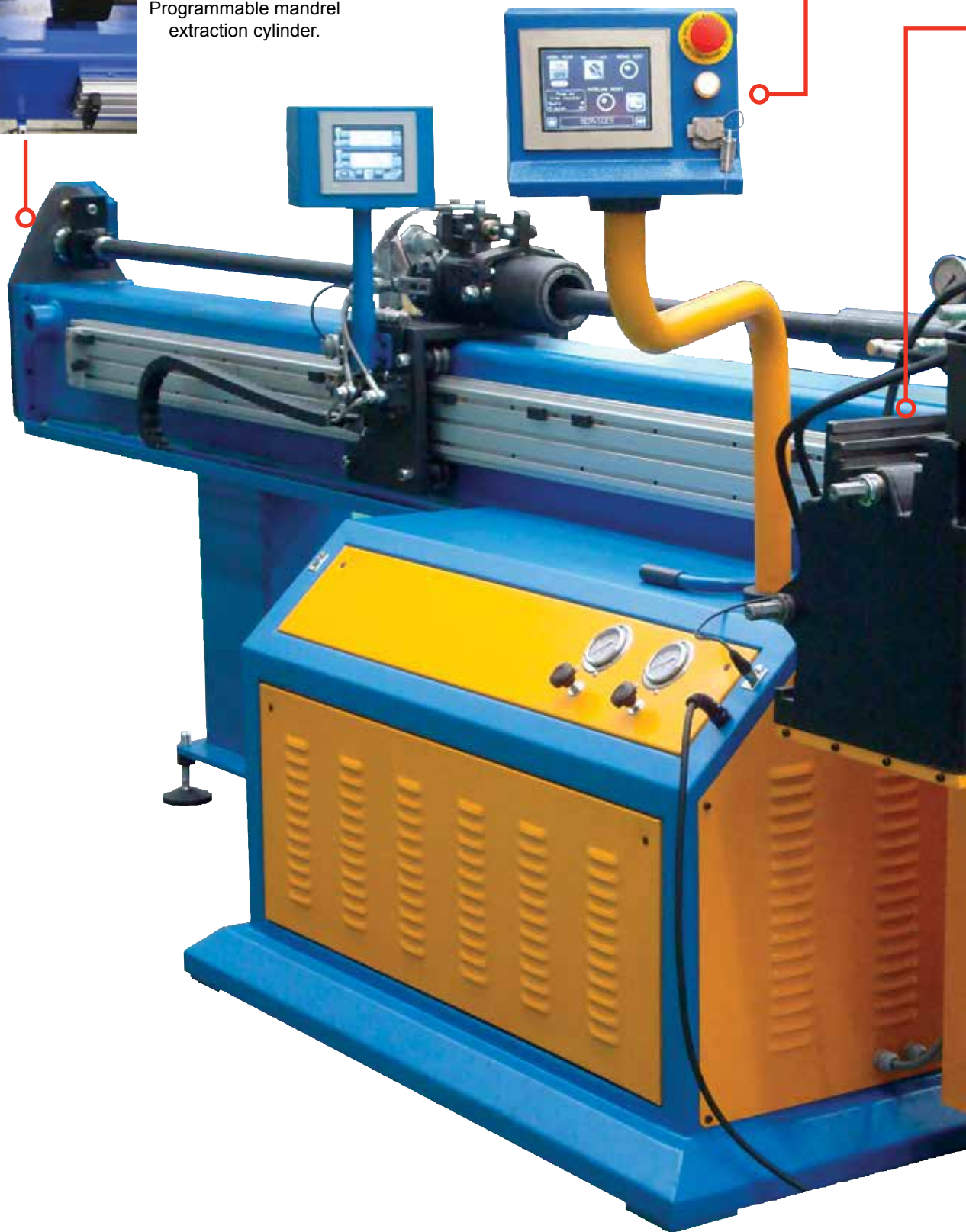
Touch screen with USB unlimited program storage.
