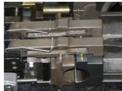
Patented finger style (FST) clamping system minimizes clamping area.
