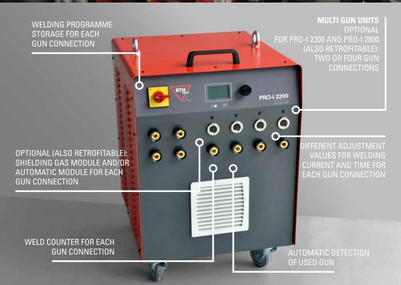
MODERN INVERTER TECHNOLOGY ENSURES VERY PRECISE CONTROL AND HIGH REPRODUCIBILITY OF THE WELDING PROCESS
