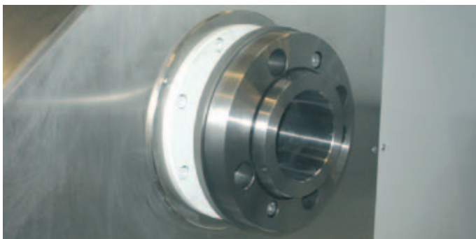
High accuracy and rigidity of the spindle by precision bearing arrangement and standard spindle bore diameter 93 mm.
