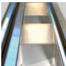
Torsion-resistant bed of high quality cast iron with hardened, fine grinded guideways and glass-scale in X-axis.
