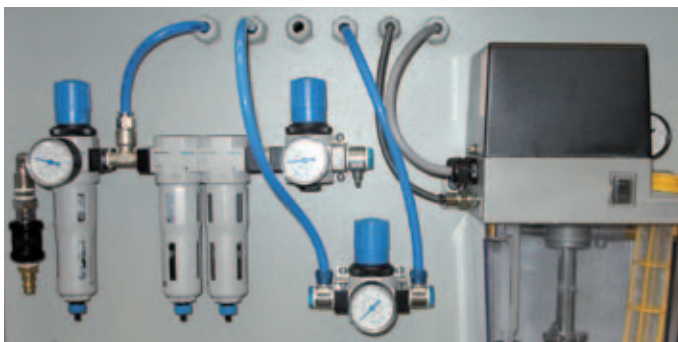
Automatic central lubrication of the guideways and nuts. Sealing air system with carbon filter for the linear measuring system in the X-axis.
