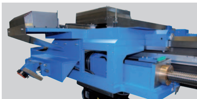
Robust apron with driven nut at a center distance of 6.000 mm.
