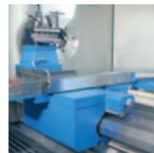
Torsion-resistant bed of high quality cast iron with hardened, fine-grinded guide-ways and glass-scale in X-axis, apron guide-ways as additional reinforcement at the front.
