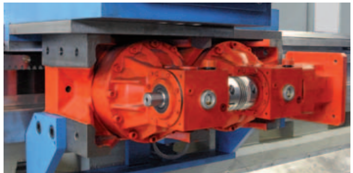
At a center distance starting with 6.000 mm a solid rack and a gear with gear wheels tensed against each other.
