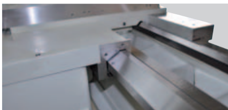
Solid saddle with plastic laminated counter guidance at the support. Long continuous cross slide with adjustable V-ledge. Cross slide guidings hardened.
