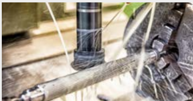
Milling of drive roll
