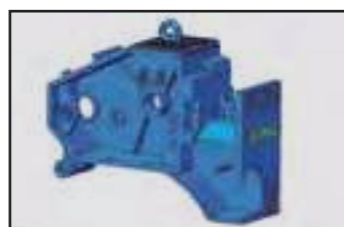
Heavy cast-iron monoblock chassis.
