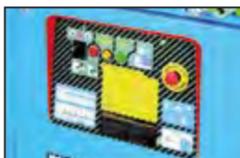
Protection shield for control panel.
