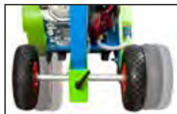
Rear tubeless puncture-proof wheels and adjustable axle.
