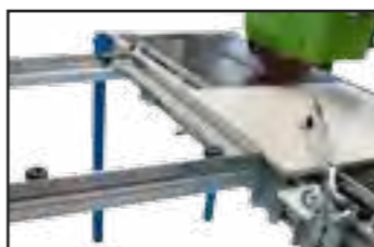
Side support with two clamps, improves precision while cutting (optional).
