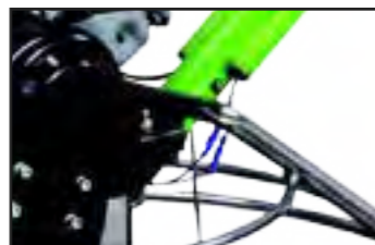
The triple tube arm is removable. Inside, the electric wiring and the accelerator.
