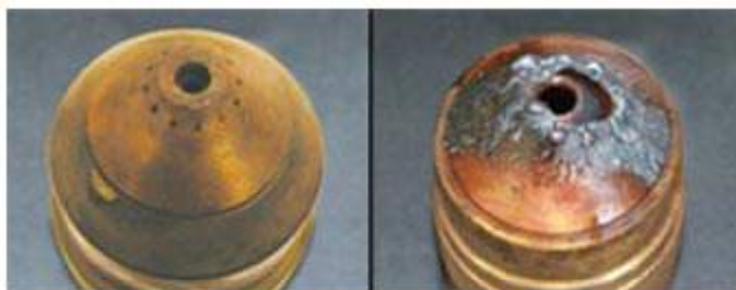
300 pierces at 50 mm (2") HPR400XD with PowerPierce technology
