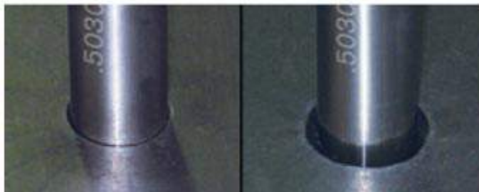
12 mm (1/2") hole with True Hole technology
