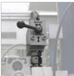
PRESSURELESS LOWERING of upper welding attachment via manual valve at the cylinder
