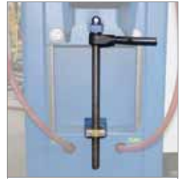
ADJUSTMENT DEVICE with ratchet for height adjustment of bottom fitting
