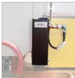
RETURN STROKE MONITORING electrical operated
