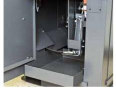
Big front door for good accessibility for saw blade changes and disposal of swarf.
