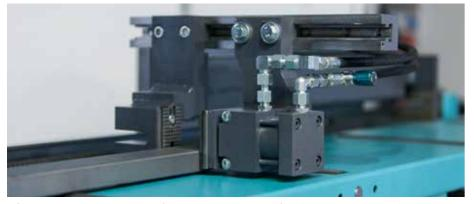
Infeed measuring device **M 45 NC** for the automatic material feed (KKS 400H/KKS 450 H). Alternativally used as a NC-controlled length stop. The M 45 NC clamps the material at the bar end and is driven forward automatically according to the programmed length.
