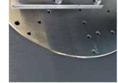
Drilling pattern in the saw table to enter fixtures of the customer's own design.
