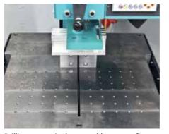
Drilling pattern in the saw table to enter fixtures of the customer's own design.
