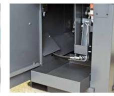
Big front door for good accessibility for saw blade changes and disposal of swarf.
