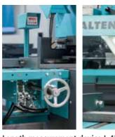
**Length measurement device L 45 I** The adjustment of the stop is controlled via hand crank and hydraulically clamped via the manual valve on the L 45 I. The digital display registers the position.
